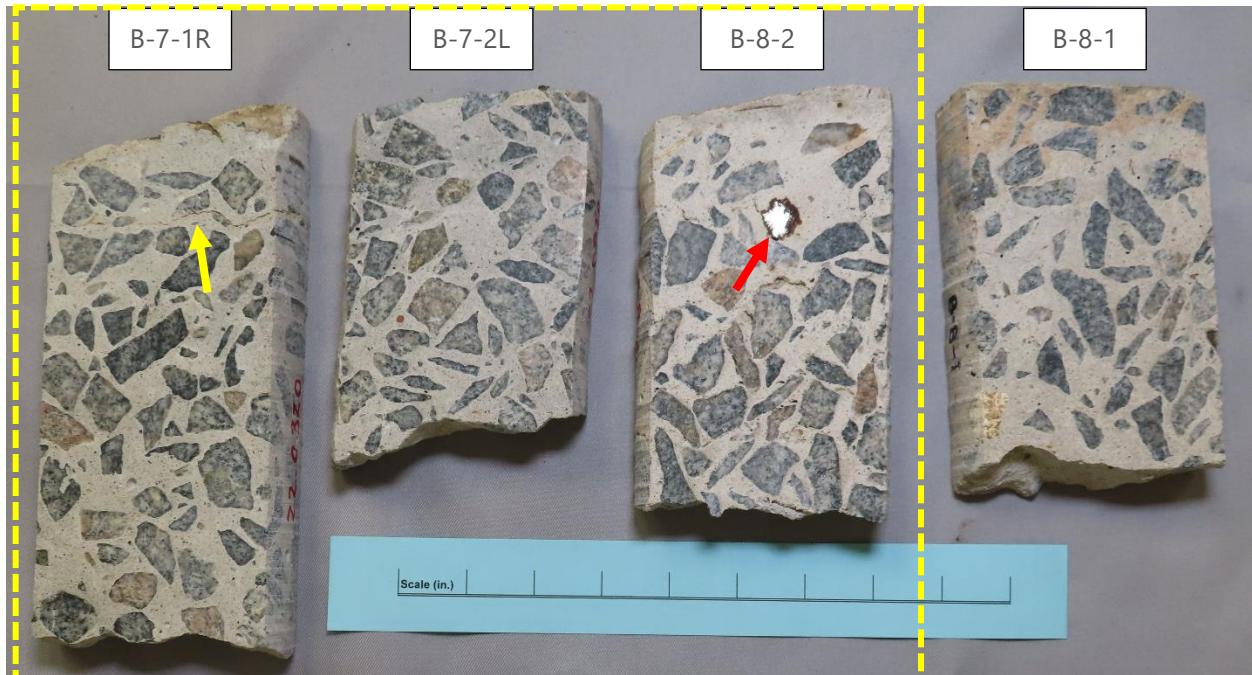
Figure A9. Lapped surfaces of the four examined core samples with compositionally similar concrete constituents. Variability in the volume and distribution of aggregates is apparent. The cores in the boxed region were extracted from within the waterline fluctuation zone, and Core B-8-1 was extracted at a higher elevation. A separation is identified with a yellow arrow in Core B-7-1R. A reinforcing bar intersected by Core B-8-2 is identified with a yellow arrow. The pink paste discoloration along the exterior surface (to top of the image) of Core B-8-1 is due to carbonation.
