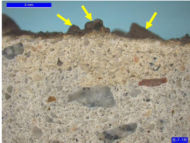
Figure 4. Aggregates (arrows) protruding from the exterior surface.
